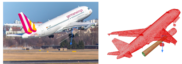
Fig. 1. An acoustic wave (blue arrow) emitted by the aircraft’s engine, reflected on the wing and crossing the jet flow. Real-life case (left) [6] and a numerical model example (right). The red surface mesh represents the aircraft’s surface and the surface of the green volume mesh of the jet flow.
