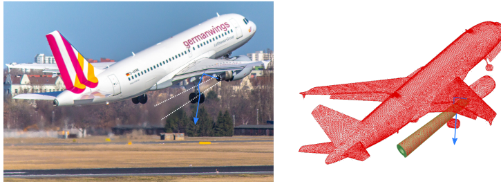
FIGURE 1: An acoustic wave (blue arrow) emitted by the aircraft's engine, reflected on the wing and crossing the jet flow. Real-life case (left) [25] and a numerical model example (right). The red surface mesh represents the aircraft's surface and the surface of the green volume mesh of the jet flow.
